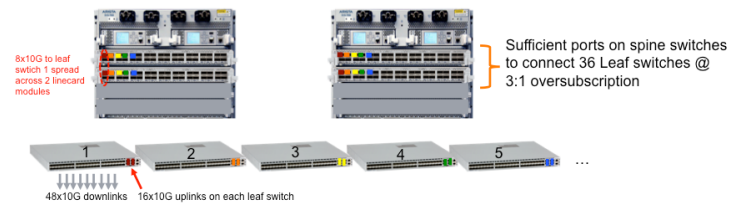
Figure 7: First expansion of spine in a scale-out design: second linecard module
